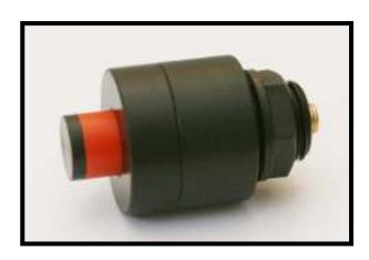
This Indicator is used as a quick and reliable visual indication of the status of a pneumatic system. The unit shows red when pressurised and is designed to be panel mounted. A 4mm push in connection aids speedy assembly and requires no special tools. By removing the internal spring this unit becomes a memory indicator showing the last signal received.
