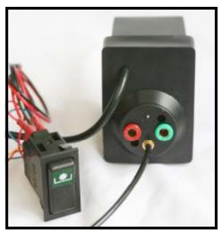
This control valve will operate a single acting PTO. Each push in fitting has a colour coded cap to ensure correct installation. The control valve is encased in a rigid rubber housing and is fully sealed against normal conditions expected beneath a road vehicle, this allows mounting of the unit in almost any position.
